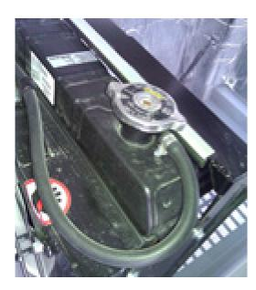
5. Check the engine liquid coolant level.
