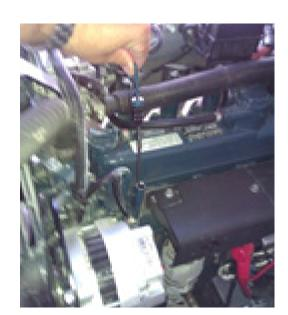
7. Check the engine oil level with the oil stick on the internal side of the engine.
