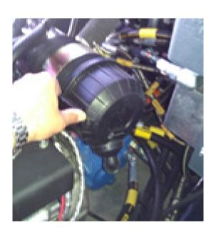
8. Make sure that the engine air cleaner and pre-filter are free from dust.
