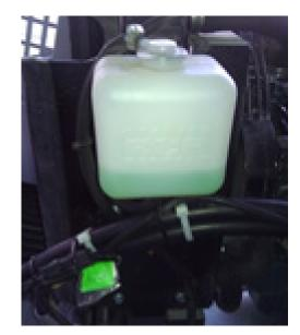
6. In case it is low check the amount of liquid in the expansion tanks and if needed use to refill the radiator.
