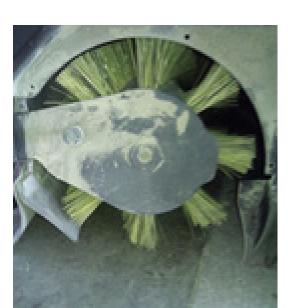
2. In case refill/change the LPG bottle. 3. Check the main broom bristles wear out and Check that the main broom freely rotate and free from ropes or debris.
