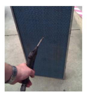
10. In case blow the filter with air.
