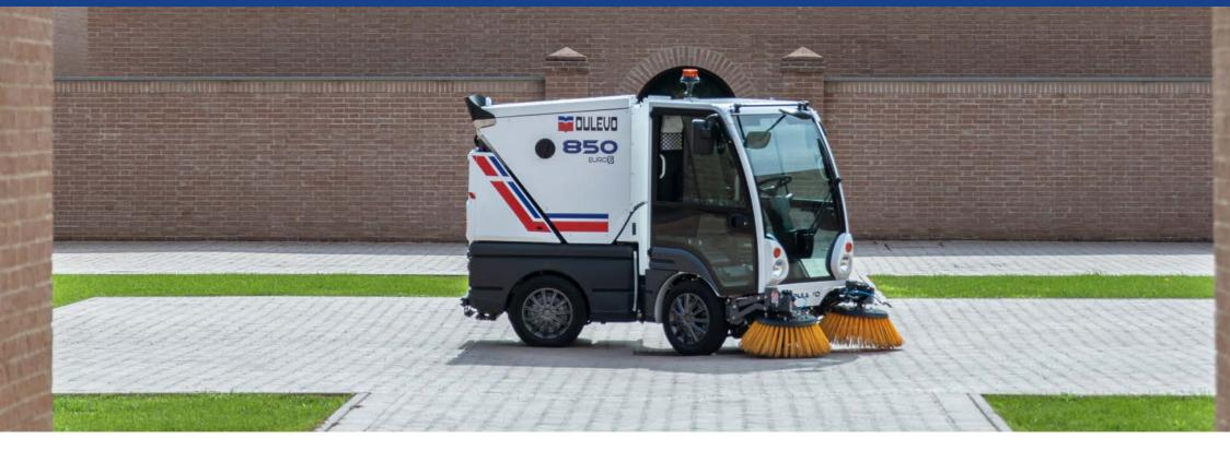
The full motion side brushes are excellent for sweeping corners, gutters and for increasing the working width. The large button window allows the operator perfect view on the suction mouth. As additional working tools a high pressure unit and a manual suction hose can be fitted optionally to enlarge the working spectrum.
