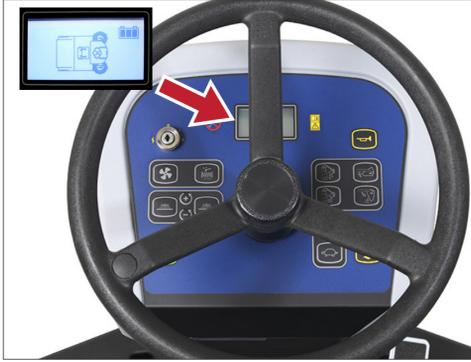
1. Check the diesel fuel tank level/LPG bottle/battery level.
