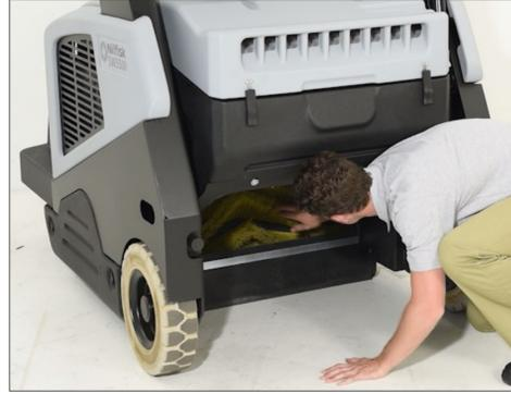
3. Check that the main broom can freely rotate and is free from ropes or debris.
