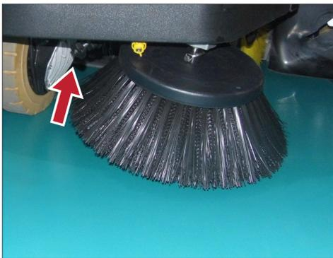
5. Check the height of side brooms and their wear condition. In case, adjust the height by rotating the knob.
