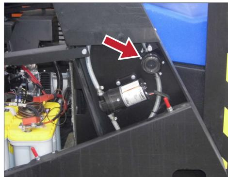
7. If the machine is equipped with DustGuard/misting system, remove the right plastic cover and check the the water filter.
