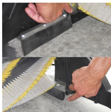
1. Check if the flaps are correctly adjusted and not worn out.
