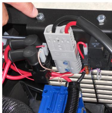
2. Check if the main battery connector is properly connected.
