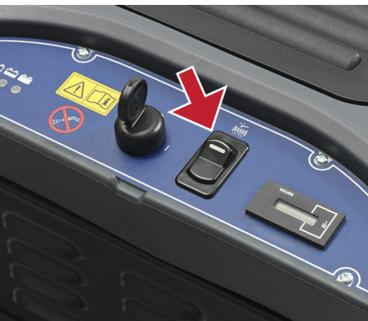
7. Activate the filter shaker switch every 10 min.
