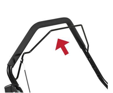
5. Activate the traction by pulling the lever.
