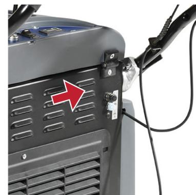
4. Check if the circuit breaker for side brooms is open.
