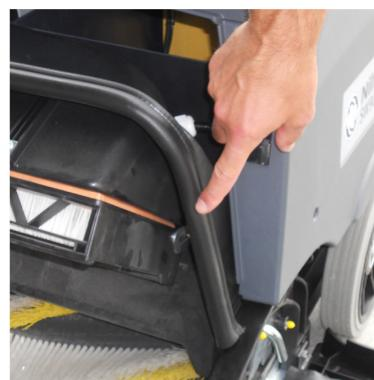
3. Check if the gasket is damaged.
