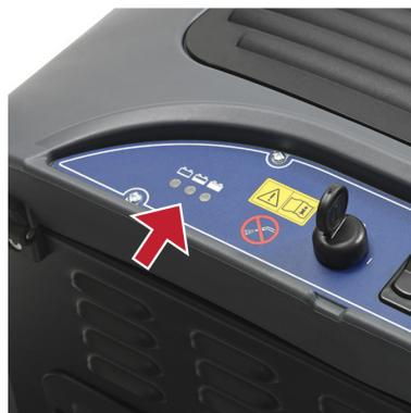
1. Check if the battery is charged and that the charger cable is disconnected from the main.
