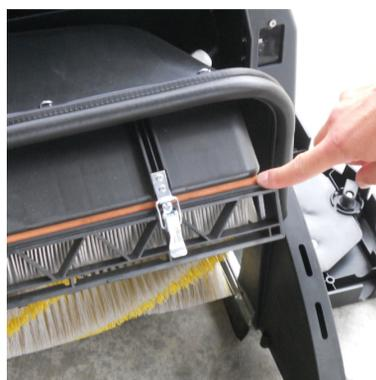
2. Check if the panel filter is clean and the gasket properly sealing.
